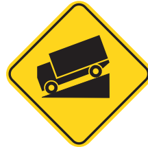
Black on yellow. Steep downgrade ahead. Slow down and shift to a lower gear to control speed and preserve brakes.
